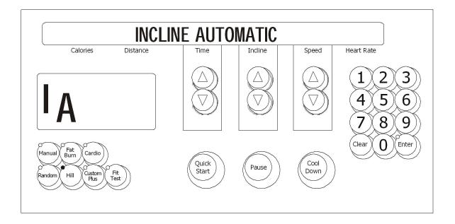
Upon entry into this test the letters IA (incline automatic) will appear in the profile window. This test allows the user to test the lift motor and switches controlling the target incline. The user can select a target incline by using the incline arrow keys. The actual incline as calculated by the time count is shown in the actual portion of the message center.
